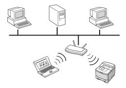
**Note**: If you connect a network cable to the Samsung Network Printer Card, the print server will not use the wireless interface. All packets will be transferred via the wired LAN.
